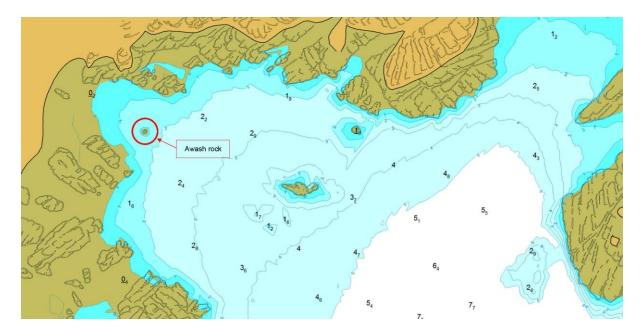
**April 2020 and June 2021: Correction to a correction!: Chart 5724A, edition 2, Lochcarron Bay:** a professional survey in early 2020 reported a 1.9m rock in an area we show as over 3m and close to a 2.8m sounding. The position is 57deg 23.78N, 5deg 28.95W. See extract from our chart, below. We reported this as a correction in April 2020. In June 2021 we re-surveyed the area to find no trace of the reported rock. The UKHO has been notified.
